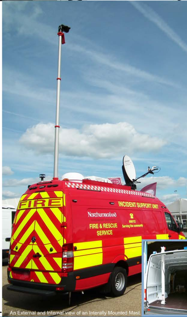
An External and Internal view of an Internally Mounted Mast
