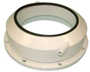
CAT NO. 14048 Roof Bearing Used when fitting a PT mast through the roof of a vehicle allows 360 degree rotation and is fitted with PTFE bearings and a weather proof ring. Weight: 1.26kg
