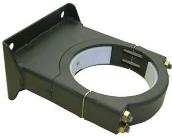
CAT NO. 14049 Upper Mounting Bracket Used to mount mast externally on a wall or shelter. Allows the mast to rotate 360 and fitted with PTFE bearing pads Weight : 2.27kg
