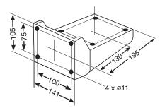
**LOWER MOUNTING BRACKET** Cat. No. 40220 Designed to receive either the fixed or rotatable base depending on the mast application. Weight: 1.59 kg.
