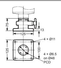
**ROTATABLE BASE** Cat. No. 40224 For use where full mast rotation is required whether internally or externally vehicle mounted, wall or shelter mounted. Fitted with clamp brake. Weight: 1.36 kg.
